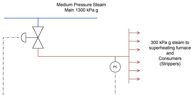
A thermocompressor can be used to withdraw some LP steam to supply these consumers. The motive stream for the thermocompressor will be MP steam. In this way the MP steam demand will be decreased.
