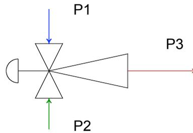
The flow ratio “suction flow/motive flow” depends on the pressures utilised. *The thermocompressor is a control valve* and can control pressures, flow rates etc as a normal control valve. The thercompressors achieve this by changing the internal nozzle pass section changing the motive stream flow rate and, consequently, the suction stream flow rate. The flow ratio varies for different valve positions.
