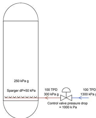
However we know that letting down steam is not the best way to use the steam. *An opportunity to generate mechanical energy is lost.* Complicated arrangements using traditional technology could be developed to meet the required intermediate pressure using a mixture of low pressure and high pressure steam generating useable mechanical energy. But although they would be technically feasible they would become *economically unacceptable* based on the capital required.
